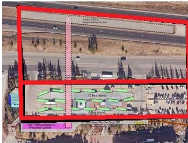
Schematic design of bus terminal and vehicular drop-off/pick-up expansion at the Vail Village Transportation Center.
